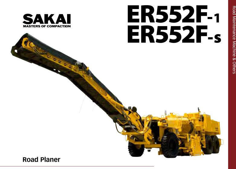
A 28 ton, fast mobilization speed milling machine. It makes milling jobs profitable, especially jobs on city roads with manholes, curbs, etc. and frequent short distance hauls.
